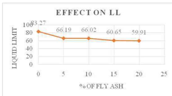
Fig 1: Liquid limit distribution curve for fly ash
