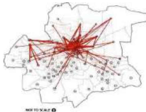
Fig. 4 Origin-destination chart with traffic analysis zones (TAZ) and desire lines (2008 Nasik CMP)
