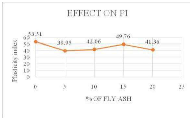
Fig 3: Plasticity index distribution curve for fly ash
