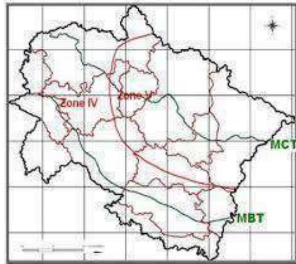
Figure 1-. Uttarakhand map showing the seismic zoning. Uttarakhand Comes under the seismic zones IV and V.
